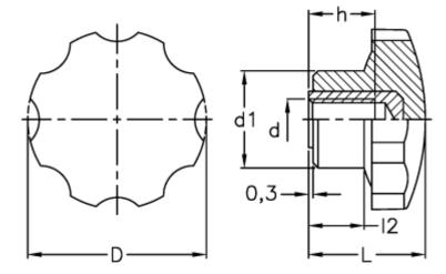
$\begin{array}{ll} D & = 54 \\ d1 & = 24 \\ d \ 6H = M8 \\ h & = 13 \\ L & = 32 \\ l2 & = 13 \end{array}$
